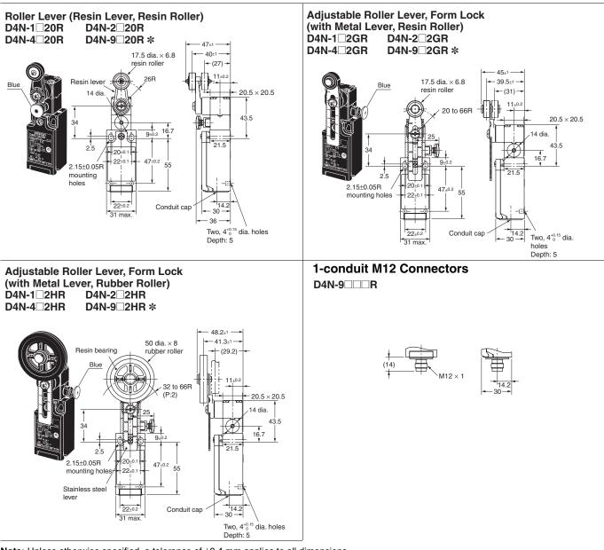
**Note:** Unless otherwise specified, a tolerance of  $\pm 0.4$  mm applies to all dimensions. \* Refer to the right above diagram for details on 1-conduit M12 connectors.
