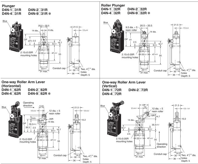
**Note:** Unless otherwise specified, a tolerance of  $\pm 0.4$  mm applies to all dimensions. \* Refer to page 7 for details on 1-conduit M12 connectors.
