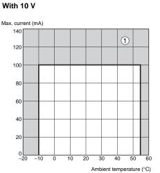
Note: 1. The above values are for standard mounting. The derating curve differs depending on the mounting conditions.
