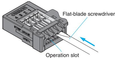
(2) Insert the wire fully to the back of the wire insertion hole. Make sure that the cable sheath is inserted into the hole, and that the end of the wire has passed through the contact section.
