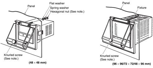
Note: Tighten the knurled screw to a torque of 0.02 N·m and the hexagonal nut to a torque of 0.05 N·m.
