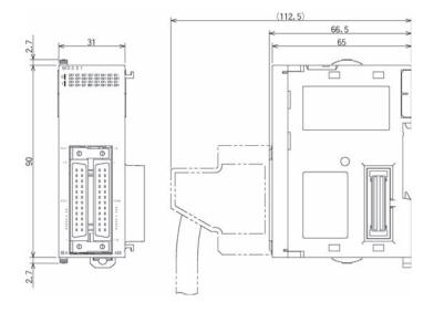
With MIL connector (20-pin  $\times$  2) CJ1W-MD232 CJ1W-MD233
