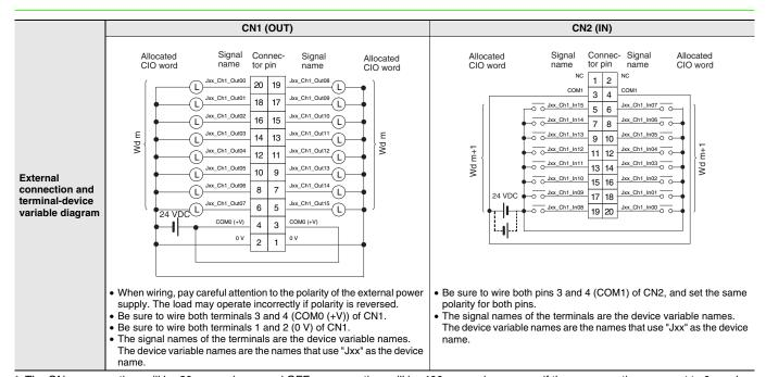
$<sup>^*</sup>$  The ON response time will be 20  $\mu$ s maximum and OFF response time will be 400  $\mu$ s maximum even if the response times are set to 0 ms due to internal element delays.
