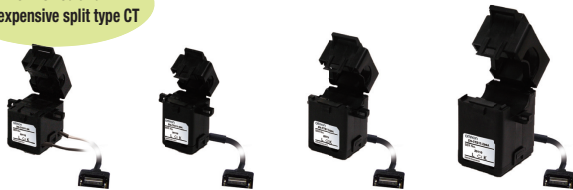
ZN-CTS11-5A Measurement range: 0.03 to 6 A CT internal diameter: 7.9mm dia. ZN-CTS11-50A Measurement range: 0.3 to 60 A CT internal diameter: 9.5mm dia. ZN-CTS11-100A Measurement range: 0.6 to 120 A CT internal diameter: 14.5mm dia. ZN-CTS11-200A Measurement range: 1.2 to 240 A CT internal diameter: 24.0mm dia.
