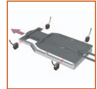
Measuring Car Body Widths (ZS-HLDS10)
