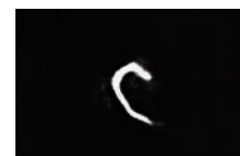
White scratch on shaded hairline finish
