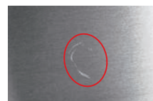
White scratch on shaded hairline finish
