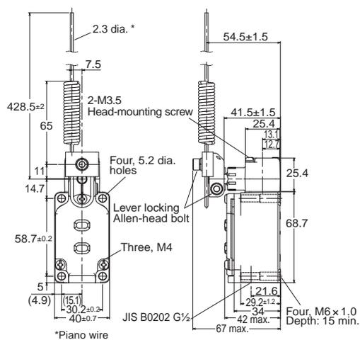
**Note:** Unless otherwise indicated, a tolerance of  $\pm 0.4$  mm applies to all dimensions.
