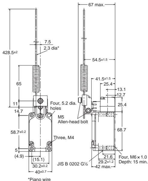
Rod spring lever With operation indicator
