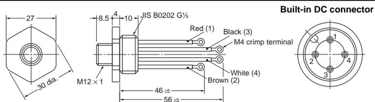
Note: 1. Each dimension has a tolerance of  $\pm 0.4$  mm unless otherwise specified.
