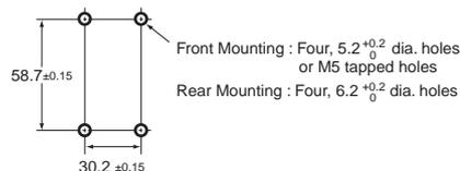
\* If the conduit size and ground terminal specifications are "with TS 1/2-14NPT ground terminal", the back mounting hole is 4-6.2 dia. <sup>+0.2</sup>/<sub>0</sub>.
