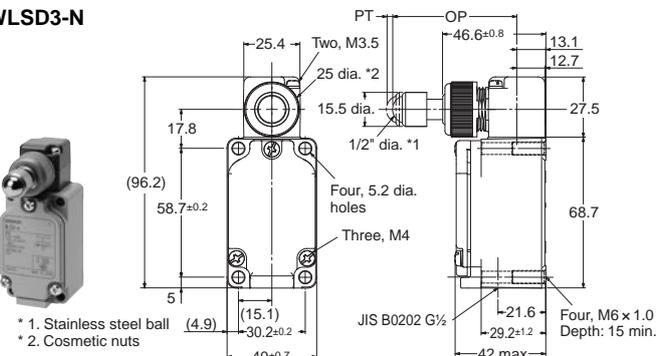
Horizontal-ball plunger With operation indicator
