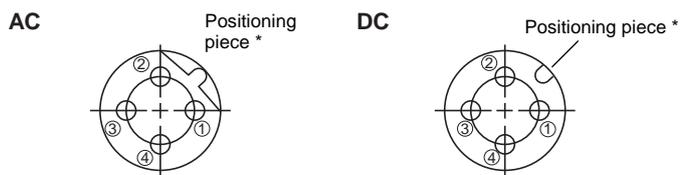
\* The position of the positioning piece is not always the same. If using an L-shaped connector causes problems in mounting, use a straight connector.
