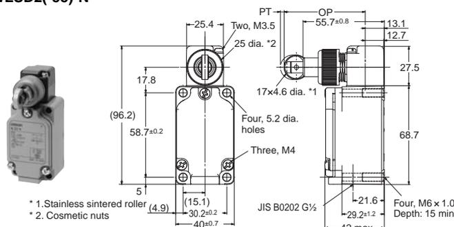
Horizontal-roller plunger With operation indicator
