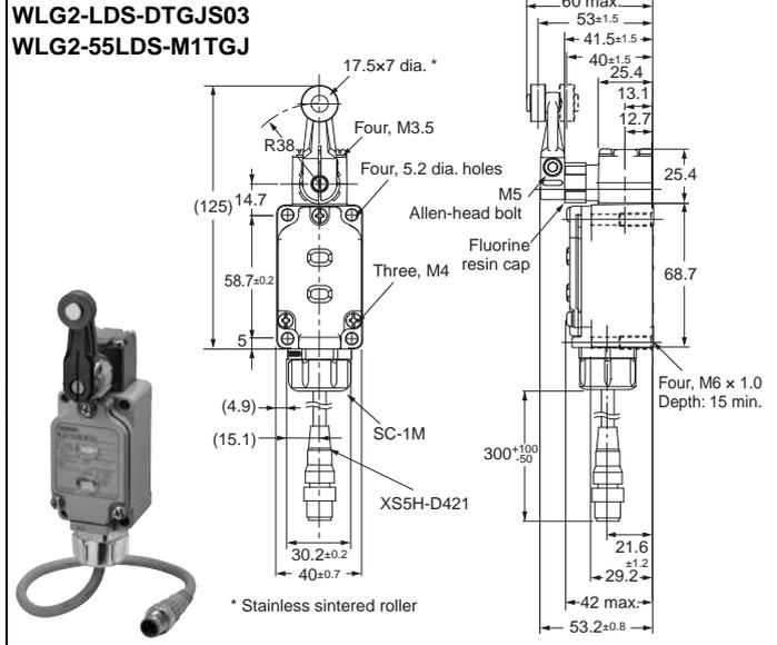
Note: The photo shows the WLG2-55LDS-M1TGJ model.
