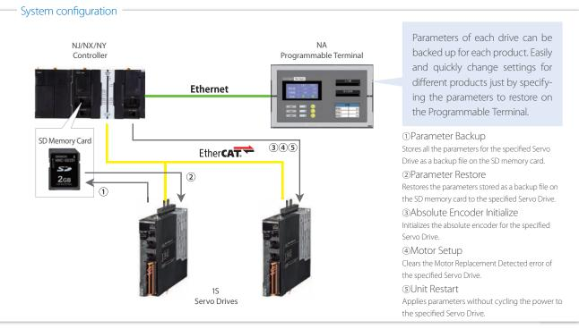
\* The Backup and Restore functions of the NJ/NX CPU Unit and the NY IPC Machine Controller can back up and restore the parameters for all the nodes at once. The addition of this library allows you to back up and restore the parameters for each node individually.
