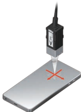
Level difference measurement of logos
