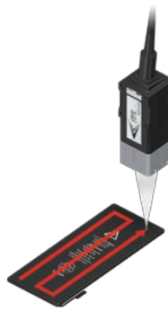
Flatness measurement of batteries
