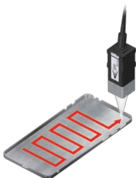
Flatness measurement of cases
