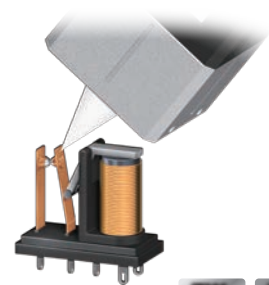
Operation inspection of relay contacts
