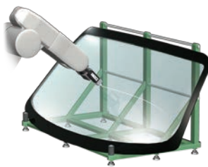
Curvature measurement of glass surfaces
