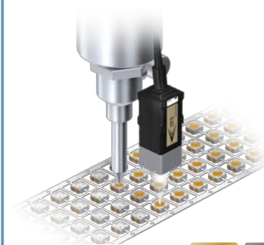
LED potting shape measurement
