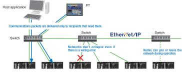
Star topology using Ethernet switch technology
