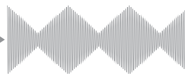
The image of the leakage current waveform at the secondary side of an inverter.
