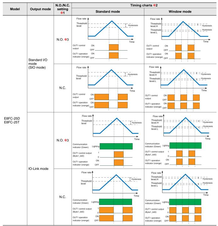
**<sup>\*1.</sup>** The N.O./N.C. setting can be changed by the operation buttons or IO-Link communications.
