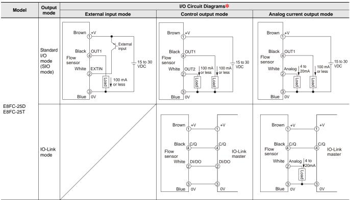
\*Pin 2 input/output can be switched with either the operation buttons or the IO-Link communication command "Pin 2 switching mode selection".
