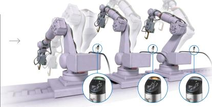
You can simultaneously monitor whether the cooling water for the welder transformer has both a "optimum flow rate" and "optimum temperature", for continuous monitoring of the cooling water performance state. This enables to detect abnormality signs of equipment.
