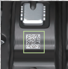
Reading direct part marks
