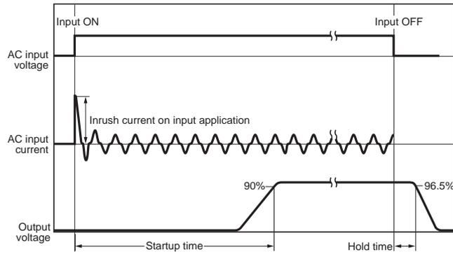
**Note:** Twice the normal inrush current will flow during parallel operation or for backup operation. Therefore, check the fusing characteristics of fuses and operating characteristics of breakers making sure that the external fuses will not burn out and the circuit breakers will not be activated by the inrush current.
