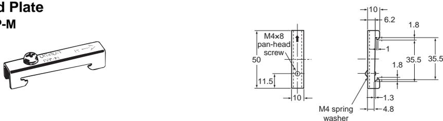
Note: 1. If there is a possibility that the Unit will be subject to vibration or shock, use a steel DIN Rail. Otherwise, metallic filings may result from aluminum abrasion.
