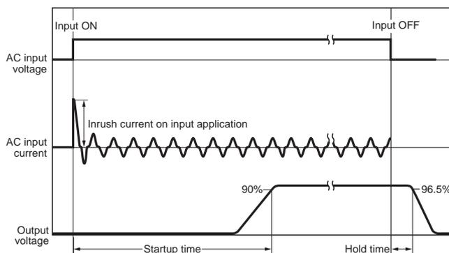
**Note:** Twice the normal inrush current will flow during parallel operation or for backup operation. Therefore, check the fusing characteristics of fuses and operating characteristics of breakers making sure that the external fuses will not burn out and the circuit breakers will not be activated by the inrush current.
