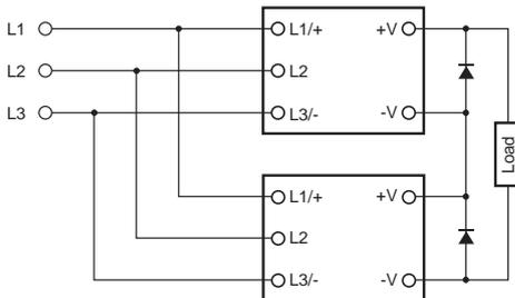
**Note: 1.** If the load is short-circuited, a reverse voltage will be generated inside the Power Supply. If this occurs the product may possibly deteriorate or be damaged. Always connect a diode as shown in the figure. Select diodes with the following ratings.
