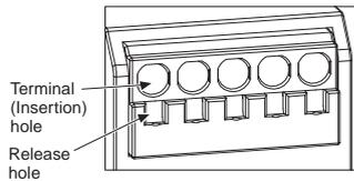
**Connecting Wires with Ferrules and Solid Wires**
