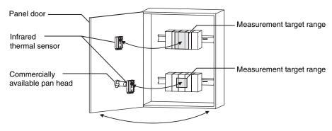
• Installing on the internal side surface of the panel by using a commercially available pan head
