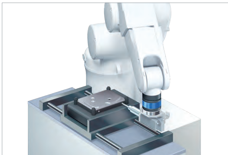
Screwing in horizontal direction
