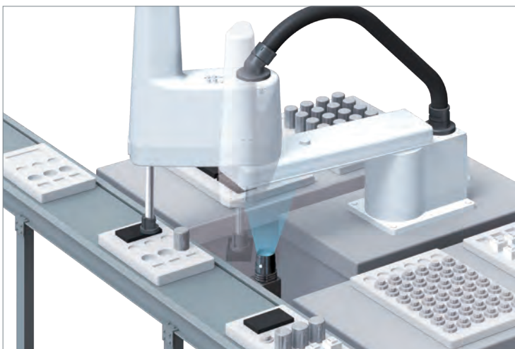
Pick & Place with position correction
