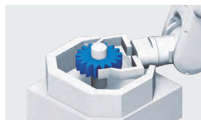
Mating requiring trial and error, including in amount of force
