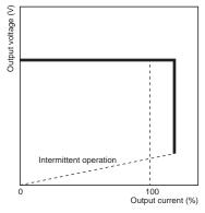
Note: 1. Internal parts may occasionally deteriorate or be damaged if a short-circuited or overcurrent state continues during operation. Be sure to check that the lout > 100% indicator is not lit or the lout > 100% signal output is turned OFF before using.
