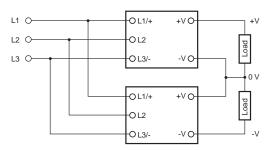
Depending on the model, internal circuits may be damaged due to startup failure when the power is turned ON if loads such as a servomotor or operational amplifier may operate in series.
