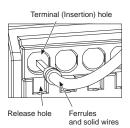
If a wire is difficult to connect because it is too thin, use a flat-blade screwdriver in the same way as when connecting stranded wire.
