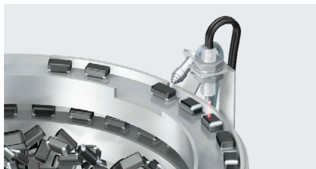
Air blower output during chip's front/rear detection
