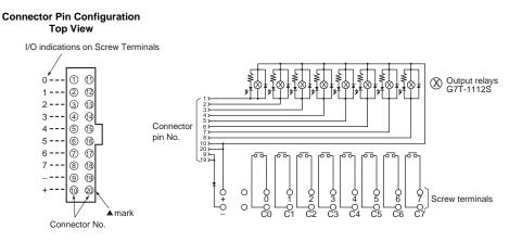
Note: Pin numbers are indicated for convenience. The ▲ mark can be used to determine orientation.
