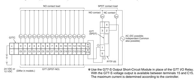
Note: If more than one G77-S Output Short-Circuit Module is employed, the voltage output of the terminals on the G7TC is as follows: G7TC-OC16: The positive side (the lower row) connects to the common line internally. G7TC-OC16-1: The negative side (the upper row) connects to the common line internally.
