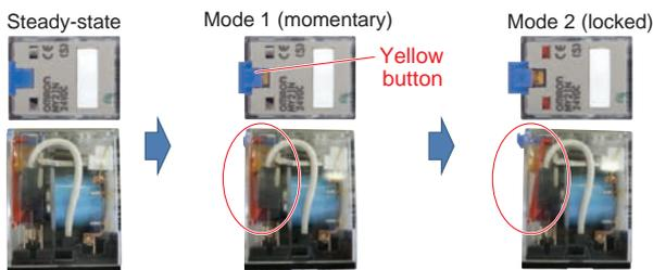
Sliding the lever to the first stage and pressing the yellow button using an insulated flat-blade screwdriver, etc., will operate the contacts.
