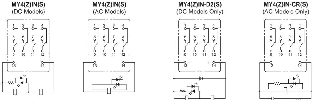
**Note:** For the DC models, check the coil polarity when wiring and wire all connections correctly.
