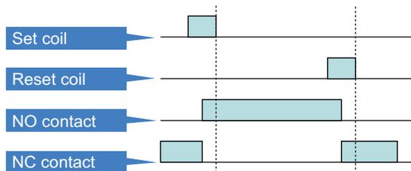
NO contact turns on when voltage is applied to the set coil and stays on even if voltage stops being applied to the set coil. NO contact turns off when voltage is applied to the reset coil, after which NC contact will turn on.\*
