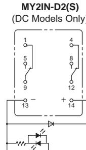
**Note:** For the DC models, check the coil polarity when wiring and wire all connections correctly.
