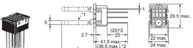
\*1. PY14QN-Y□ and PY14QN2-Y□ include the portion indicated by broken line.
