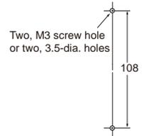
**Note:** Pull out the hooks to mount the Socket with screws.
