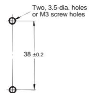
The above figure is for the MY4F. The 2-pole and 3-pole models conform to these dimensions.
